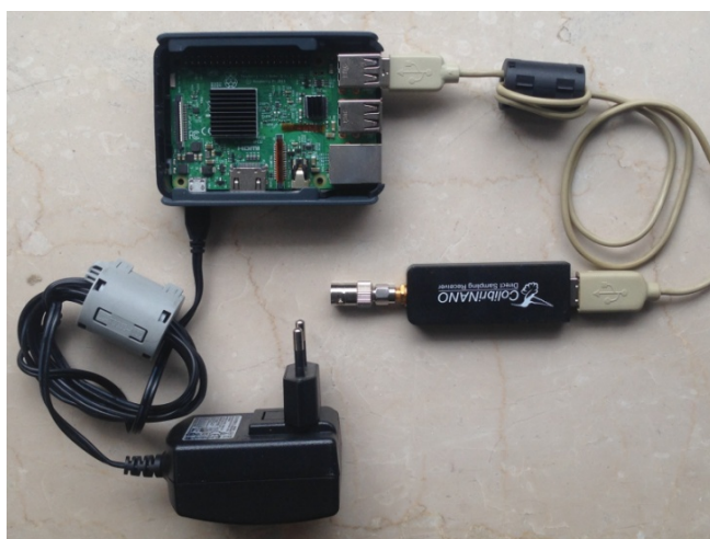
Picture 15: Direct sampling SDR receiver with RPi3 as server
