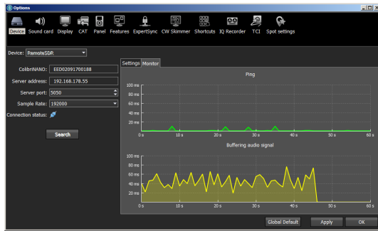
Picture 9: Entering the server address and server port
