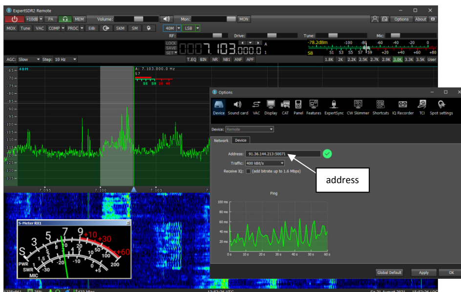
Figure 8: After entering the URL, the SunSDR2 DX can be reached worldwide via the Internet.
